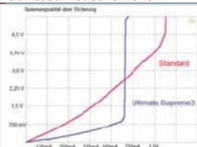
It's true: Our measurement of the voltage drop over the fuse clearly shows the internal resistance of the Supreme micro-fuse three times lower. Measured here: 250 mA fuses that burn out at about 250% of their nominal value (recognizable by the steeply rising flanks of the curves. Supreme exceeds standard fuses in conforming to normal burn out standards.
